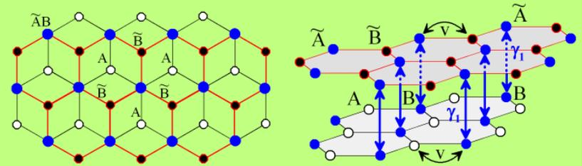
$$\mathcal{H} = \begin{pmatrix} A & \tilde{B} & \tilde{A} & B \\ 0 & 0 & 0 & v\pi^+ \\ 0 & 0 & v\pi & 0 \\ 0 & v\pi^+ & 0 & \gamma_1 \\ v\pi & 0 & \gamma_1 & 0 \end{pmatrix} \begin{pmatrix} A \\ \tilde{B} \\ \tilde{A} \\ B \end{pmatrix}$$
