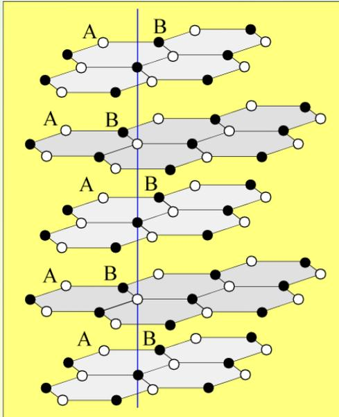
Three dimensional layered material with hexagonal 2D layers [shown here with Bernal (AB) stacking]
