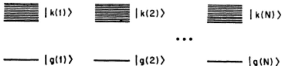
FIG. 1. Pictorial representation of photodetector consisting of  $N$ -independent atoms. Each atom in detector has a ground state  $|g\rangle$  and continuum of excited states  $|k\rangle$ . Atoms are labeled by indexing atomic state with particle number, e.g.,  $|k(m)\rangle$ .
