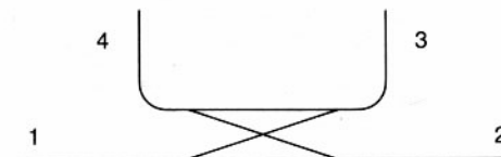
Fig. 6.21 Schematic diagram of a directional coupler.
