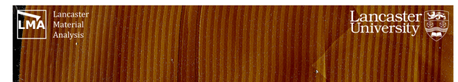
Example 7 (Vertical Cavity Surface Emitting Laser (VCSEL)). Multilayer structure of distributed GaAs/AlGaAs Bragg reflectors, with GaSb Quantum Rings in active region. Total z-scale of structure is 13 \mu\text{m} . (Sample courtesy M. Hayne, Lancaster University, UK).
